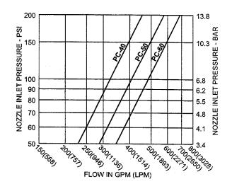
WATER OR FOAM SOLUTION NOZZLE DISCHARGE CHARACTERISTICS
