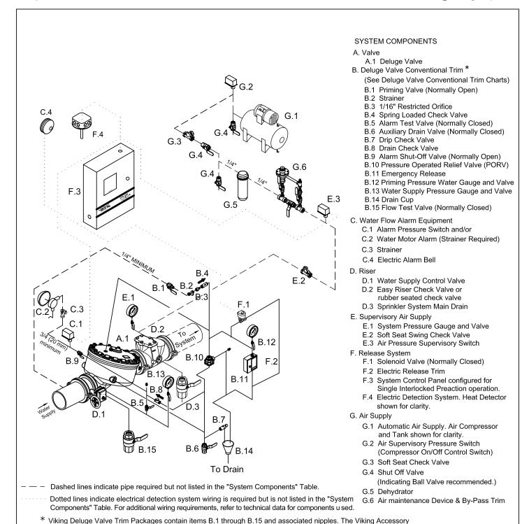
FIGURE 5: HORIZONTAL DELUGE VALVE WITH TANK-MOUNTED COMPRESSOR (6" Valve Shown)
