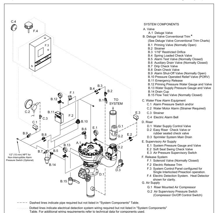
FIGURE 2: ANGLE DELUGE VALVE WITH RISER-MOUNTED COMPRESSOR (6" Valve Shown)
