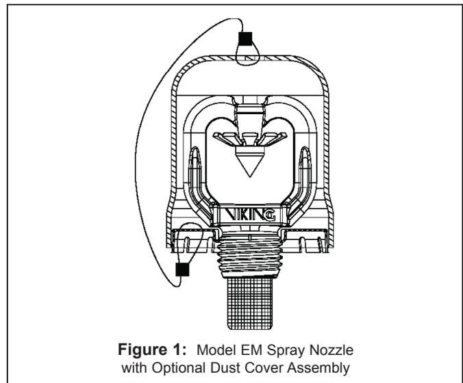
**Figure 1:** Model EM Spray Nozzle with Optional Dust Cover Assembly
