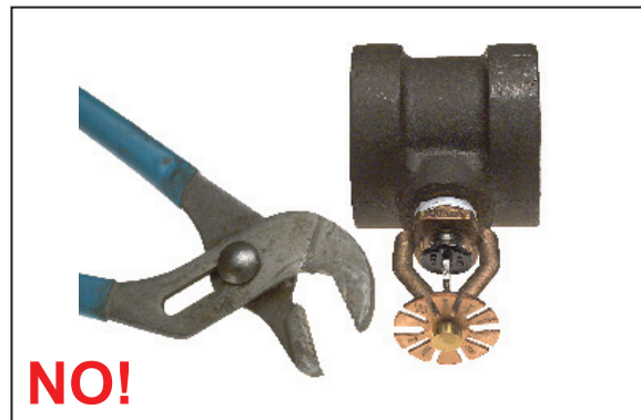
Figure 2: Incorrect installation wrench (ESFR sprinkler shown with Channel Locks)
