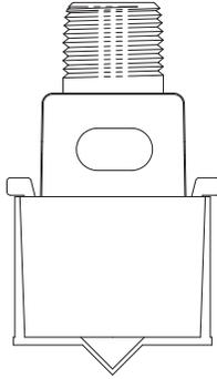
**Concealed Sprinkler Assembly with Protective Cap (Pendent Sprinkler Base Part No. 12292 shown)**
