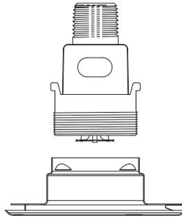
**Cover Plate Assembly (Pendent Cover Base Part No. 11697 shown)**
