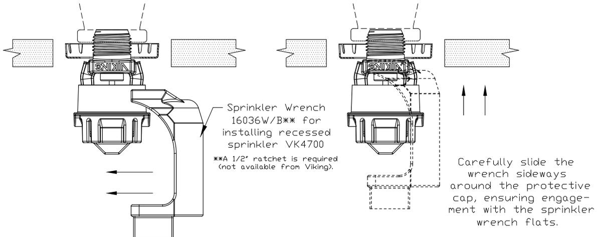
**Figure 2: Wrench 16036W/B for Installing Recessed Sprinkler VK4700**
