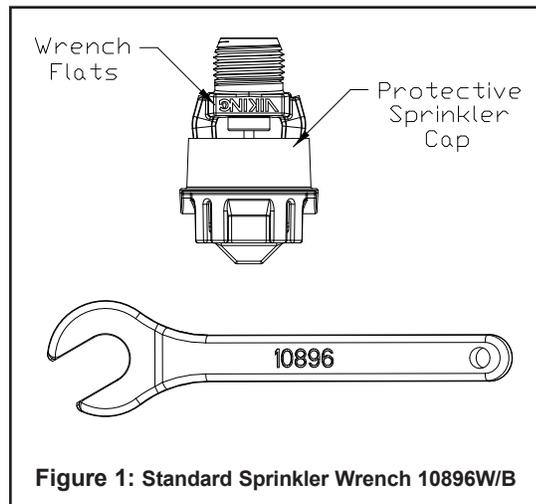
**Figure 1: Standard Sprinkler Wrench 10896WB**
