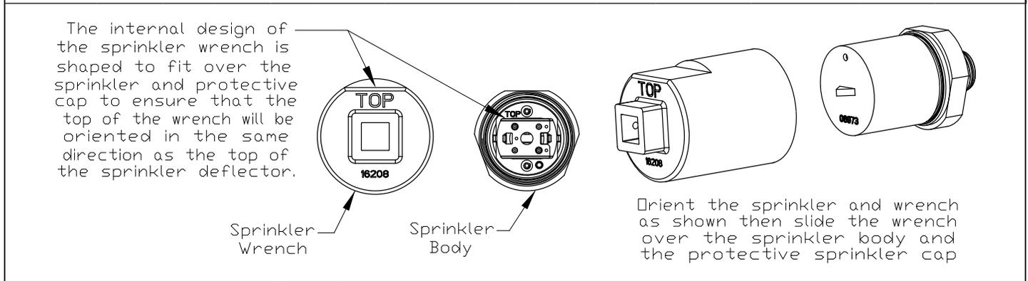
**Figure 1: Sprinkler VK481 Installation and Correct Use of Wrench**
