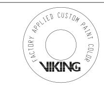
Identification of Custom Paint Color: All custom color painted cover plates will have an identifying label affixed to the inside of the cover that indicates custom color and will have a representative sample (a paint dot) of the paint on the label.
