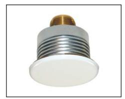
Viking Quick Response Extra-Large Orifice Sprinklers may eliminate the need for a fire pump or reduce the size of the pump if it is required. On existing systems, replacing large orifice sprinklers with extra-large orifice sprinklers may provide the higher densities required to allow an increase in the hazard classification of an occupancy.
