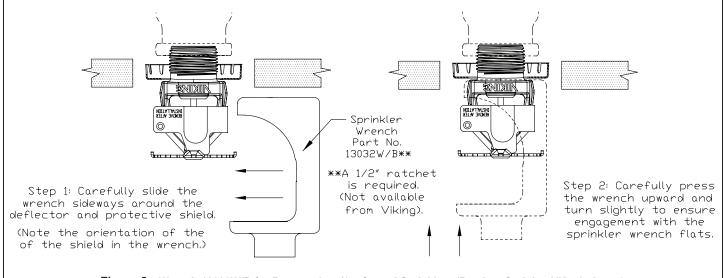
Figure 2: Wrench 13032W/B for Recessed and/or Coated Sprinklers (Pendent Sprinker VK572 shown)
