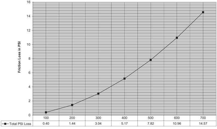
Flow in GPM (C = 120)
