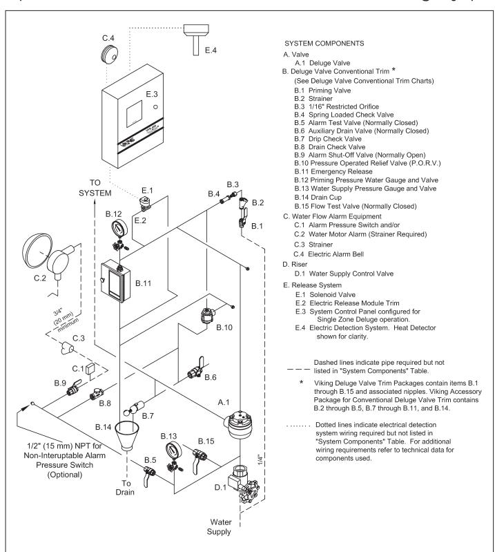
FIGURE 1: ANGLE DELUGE VALVE WITH CONVENTIONAL TRIM
