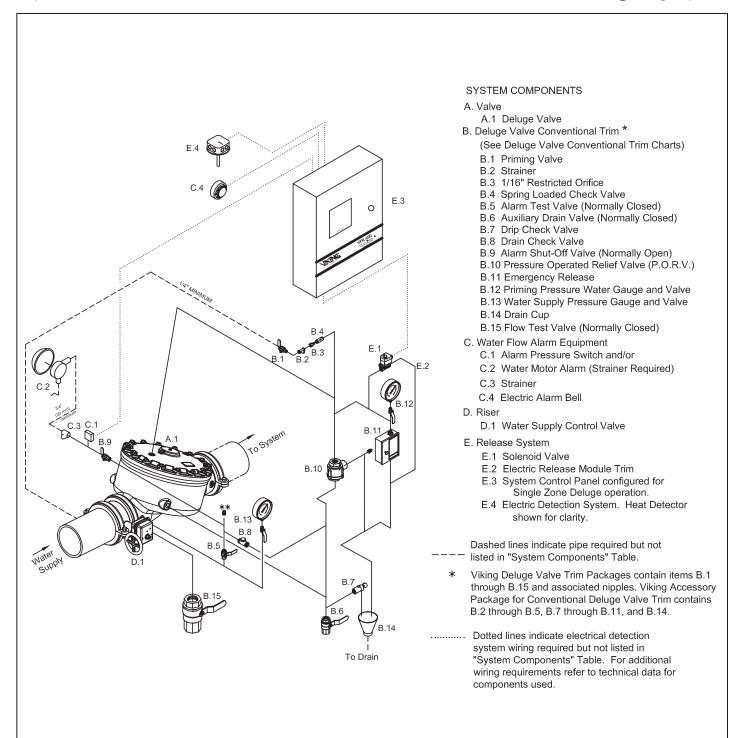
FIGURE 3: STRAIGHT THROUGH DELUGE VALVE WITH HORIZONTAL CONVENTIONAL TRIM
