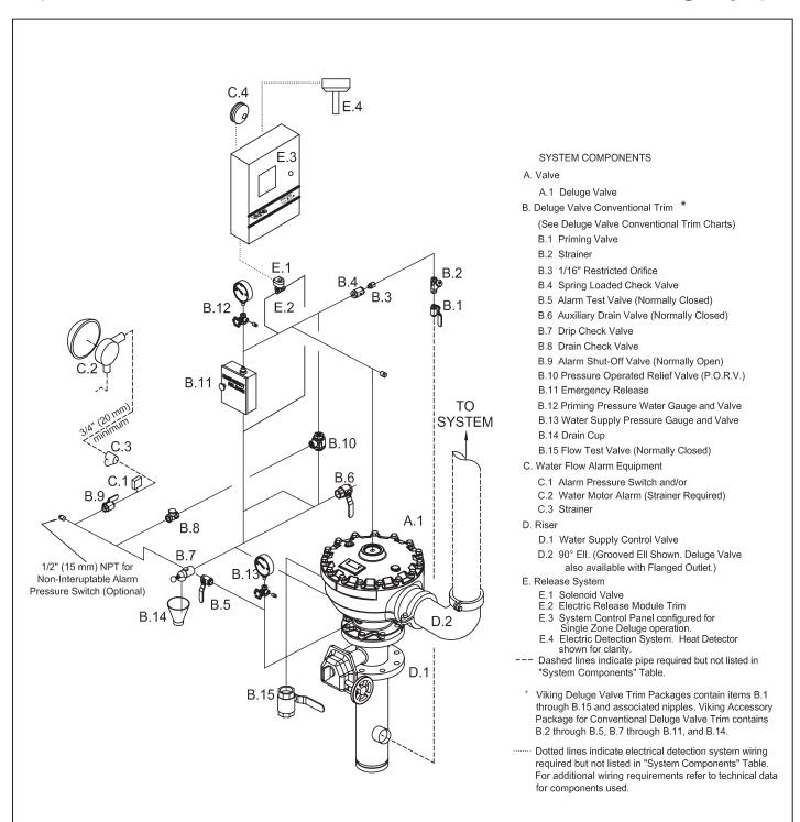
FIGURE 2: ANGLE DELUGE VALVE WITH CONVENTIONAL TRIM 6" VALVE SHOWN. ALSO AVAILABLE IN 2", 3", & 4".
