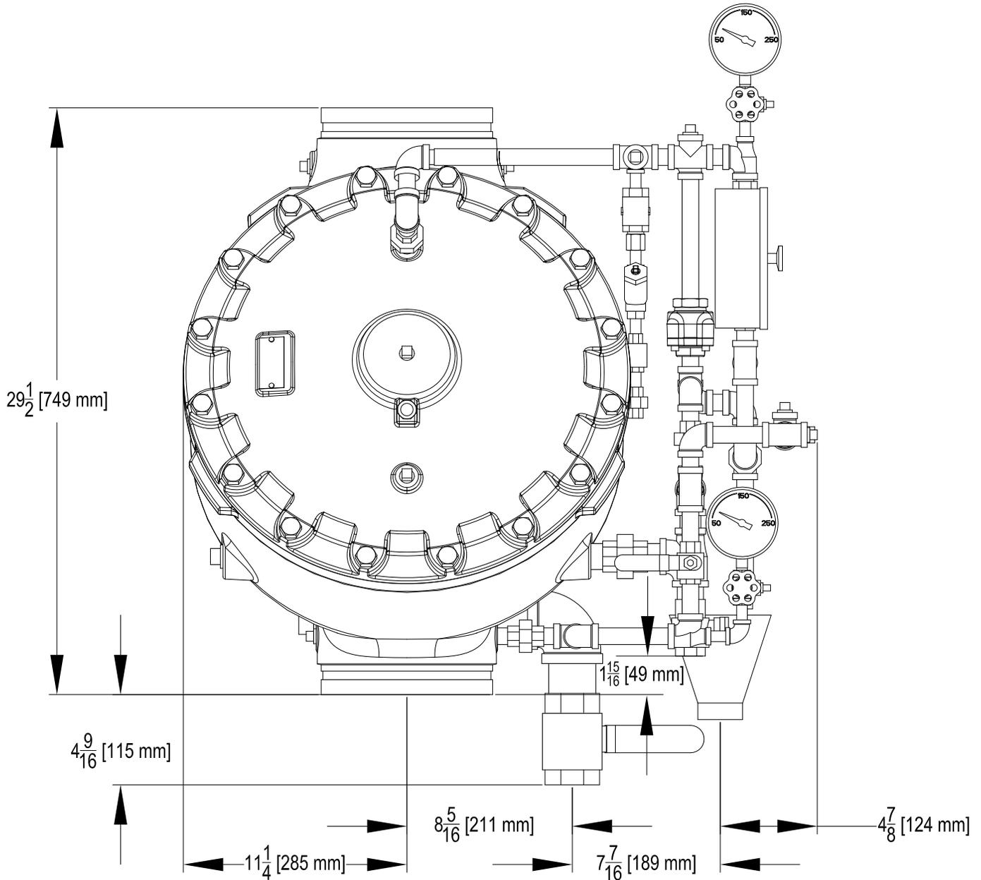
Figure 3a: Installation Dimensions
