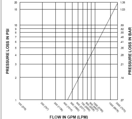
Figure 3: Pressure Loss vs. Flow F15049 Monitor
