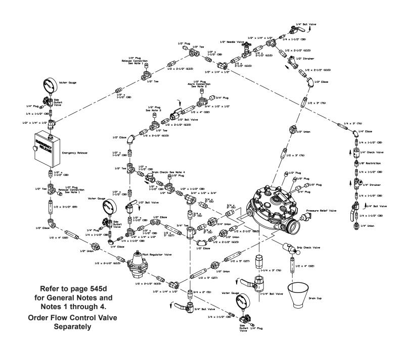
Figure 1 2-1/2" & 3" Pilot Regulating Trim for Model J Flow Control Valve
