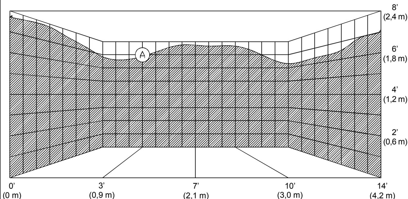
Typical profile of one half of the 14' x 14' (4,3 m x 4,3 m) spray pattern produced by a Viking Freedom™ ½" (15 mm) Residential Horizontal Sidewall Sprinkler SIN VK440 installed with the deflector located 4" below the ceiling. Nominal U.S. K-Factor = 4.3 (6,2 metric).
