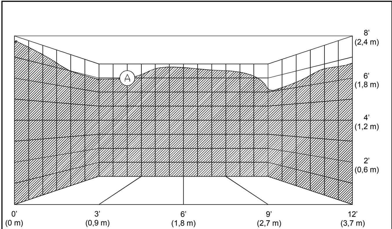
Typical profile of one half of the 12' x 12' (3,7 m x 3,7 m) spray pattern produced by a Viking Freedom™ ½" (15 mm) Residential Horizontal Sidewall Sprinkler SIN VK440 installed with the deflector located 4" below the ceiling. Nominal U.S. K-Factor = 4.3 (6,2 metric).
