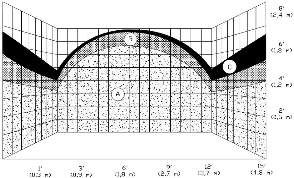
Typical profile of one half of the spray pattern produced by a Viking Model HQR-2 Institutional Pendent Sprinkler
