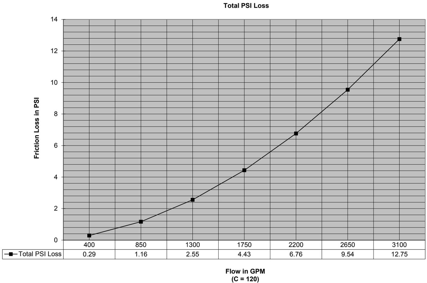
**Friction Loss for the 6" Viking Model G6000 Dry Valve is equivalent to 44.88 feet of 6" Schedule 40 (id = 6.07") Pipe (C = 120).**
