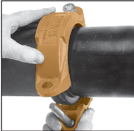
**4 HOUSINGS**— With one nut unthreaded to the end of the bolt, unthread the other nut completely and swing the coupling housing halves over the gasket, making sure the housing keys engage the grooves. Insert the bolt and turn the nuts finger tight.
