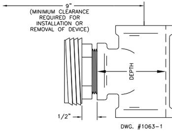
Screw the fitting into the TEE fitting as shown. On sweat TEE's, no threaded bushings, inserts or adapters are permitted unless they comply with the dimensions listed in the chart below.
