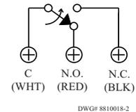
Fig. 5 Typical Electrical Connections
