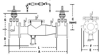
Pressure — Temperature Temperature Range: 33°F - 110°F (0.5°C - 43°C) Maximum Working Pressure: 175psi (12.1 bar)
