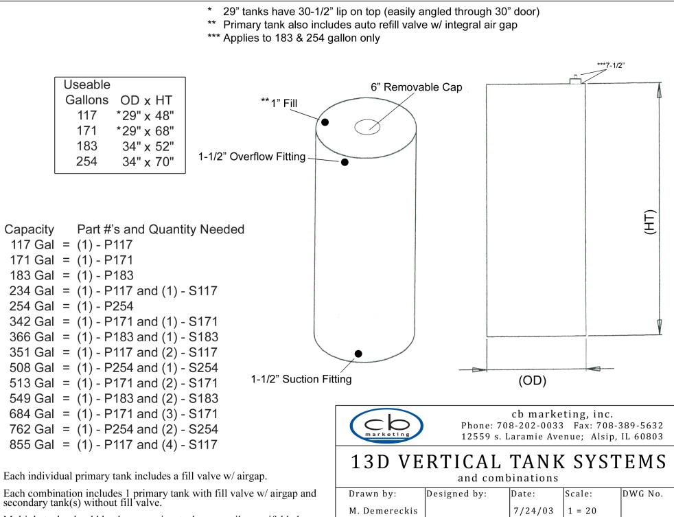
Multiple tanks should be the same size, tanks are easily manifolded.
