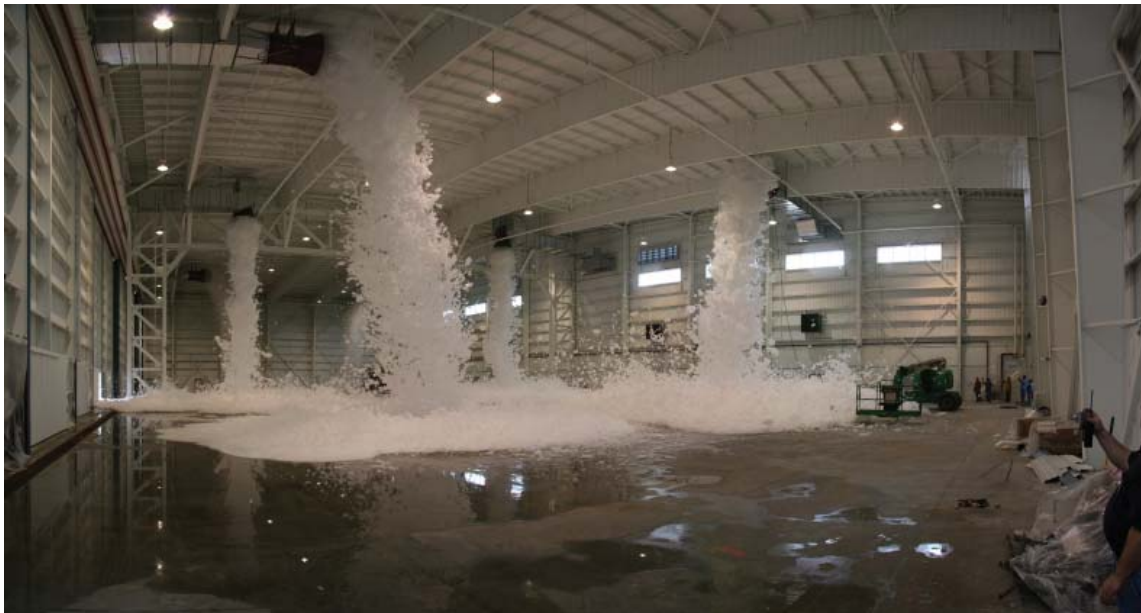
Figure 6 - Viking Foam System Testing
