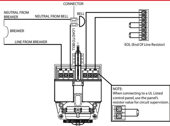
NOTE: When connecting to a UL Listed control panel, use the panel's resistor value for circuit supervision.
