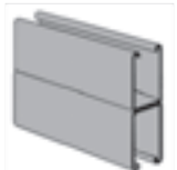
AS 150BTB WELDED CHANNEL Size: 1½" x 2½" x 12 Ga. Two Pcs. AS 150 Welded Back-to-Back
