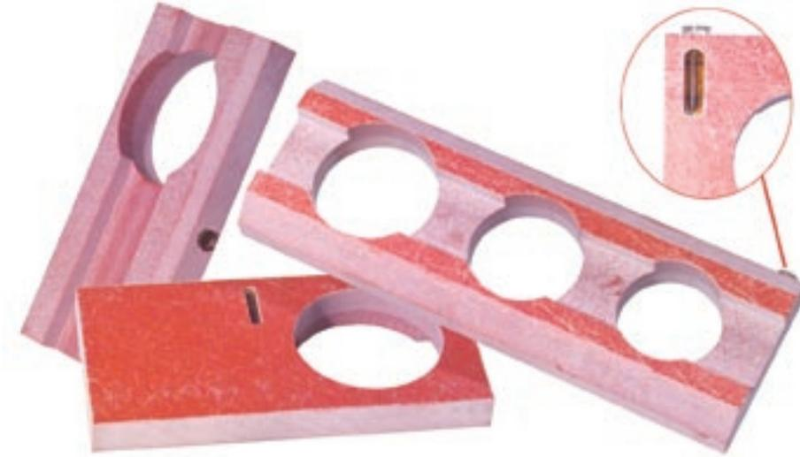
Merit® Hand-Held Hole Templates are sized to be used with air plasma cutting systems with standard torch cups measuring 1.1" (28mm) in diameter. If used with other torches, slight variations in the hole diameter required for Merit® Tee-Lets® may occur.
