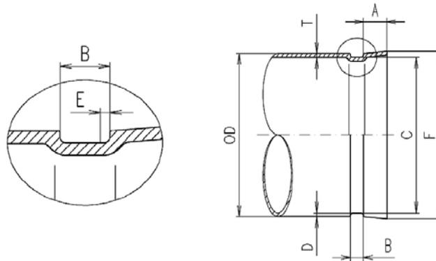
Table 14: Roll Groove Specifications for Steel pipe
