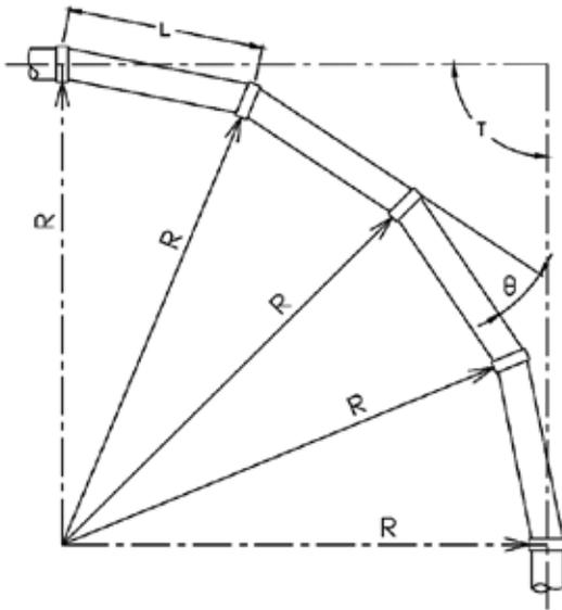
Utilizing the angular deflection at each coupling joint curves may be laid out using straight pipe lengths and Couplings.
