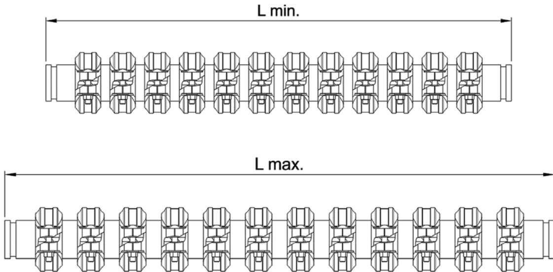
Table 12: Movement capability of couplings-expansion and contraction joints
