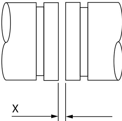
The nominal pipe end separation dimensions are suitable for system layout purposes only
