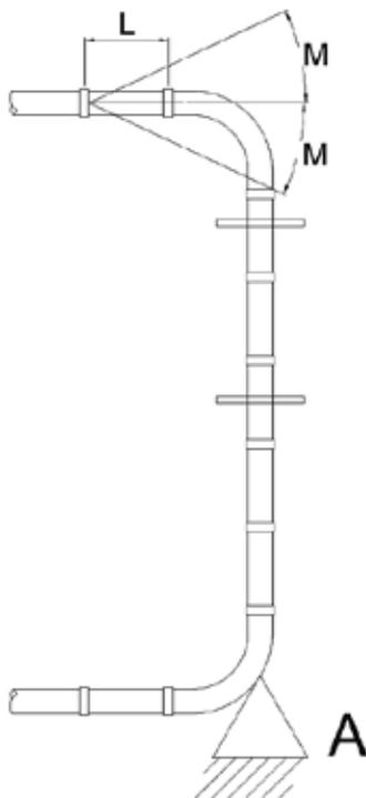
Install the riser with the pipe ends butted.
