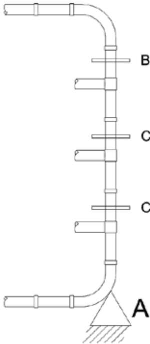
Install the riser with the predetermined gap method. Anchor the pipe at or near the base with a pressure thrust anchor "A" capable of supporting the full pressure thrust, weight of pipe and the fluid column. Anchor at "B" with an anchor capable of withstanding full pressure thrust at the top of the riser plus weight of pipe column. Place intermediate anchors "C" as shown, between anchors "A" and "B". Also place intermediate clamps at every other pipe length as a minimum.
