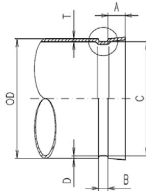
Table 15: Cut Groove Specifications for Steel pipe
