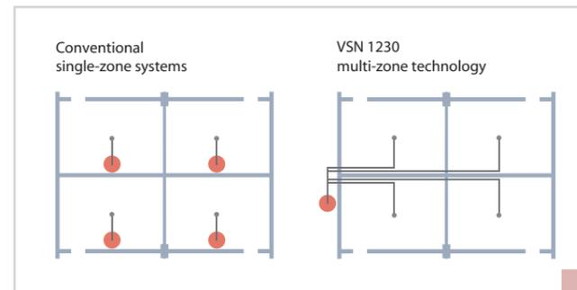
VSN 1230 fire extinguishing systems can be designed for use as a single-zone system to protect a single protected area or in the form of a multi-zone system to protect two or more areas.
