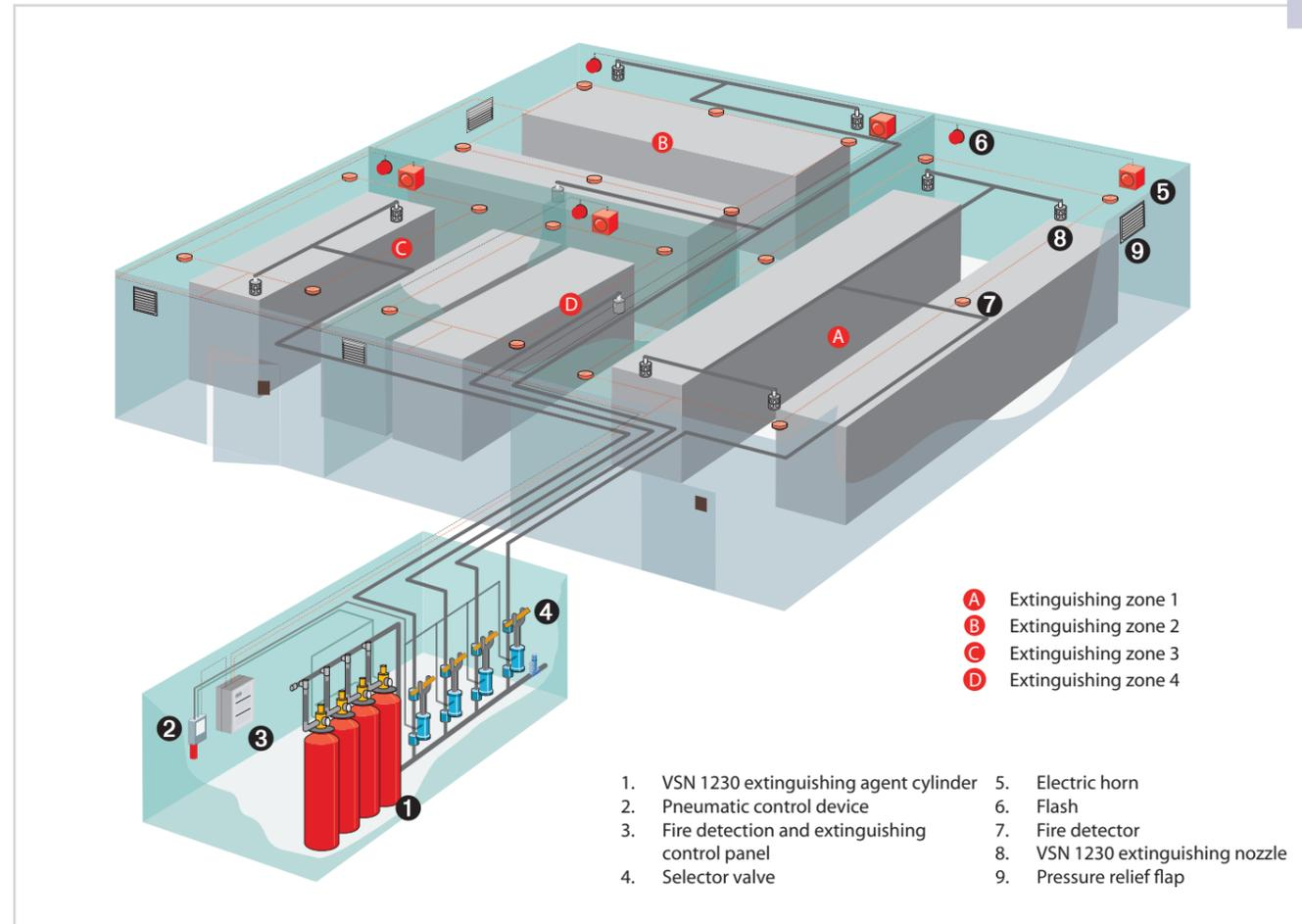
In the pipework, a two-phase flow - composed of liquid Novec 1230 and gaseous nitrogen – is generated after activation of the extinguishing system; this presents a particular challenge for the hydraulic calculation when planning the system.
