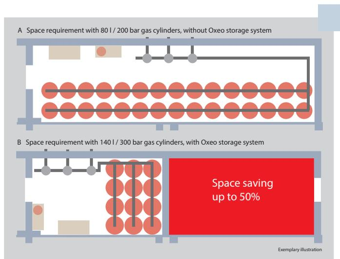
The possibility to arrange the gas cylinders in multiple rows and to adapt the cylinder setup to the premises creates additional flexibility for the inert gas storage. As a result, Oxexo extinguishing systems require up to 50% less space for the extinguishing gas supply than inert gas systems with 80 l / 200 bar gas cylinders and a conventional supply system.
