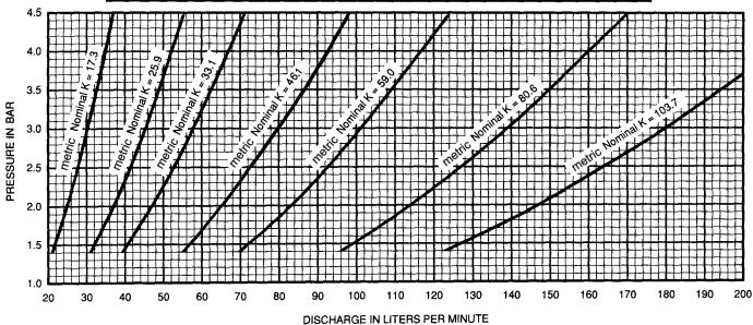
**NOTE:**  $Q = K\sqrt{p}$ ; where "Q" = flow in liters per minute, "p" = pressure in bar, and "K" is the nominal discharge coefficient.
