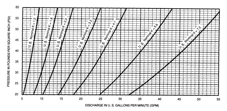
**NOTE:**  $Q = K\sqrt{p}$ ; where "Q" = flow in U.S. gallons per minute, "p" = pressure in pounds per square inch, and "K" is the nominal discharge coefficient.
