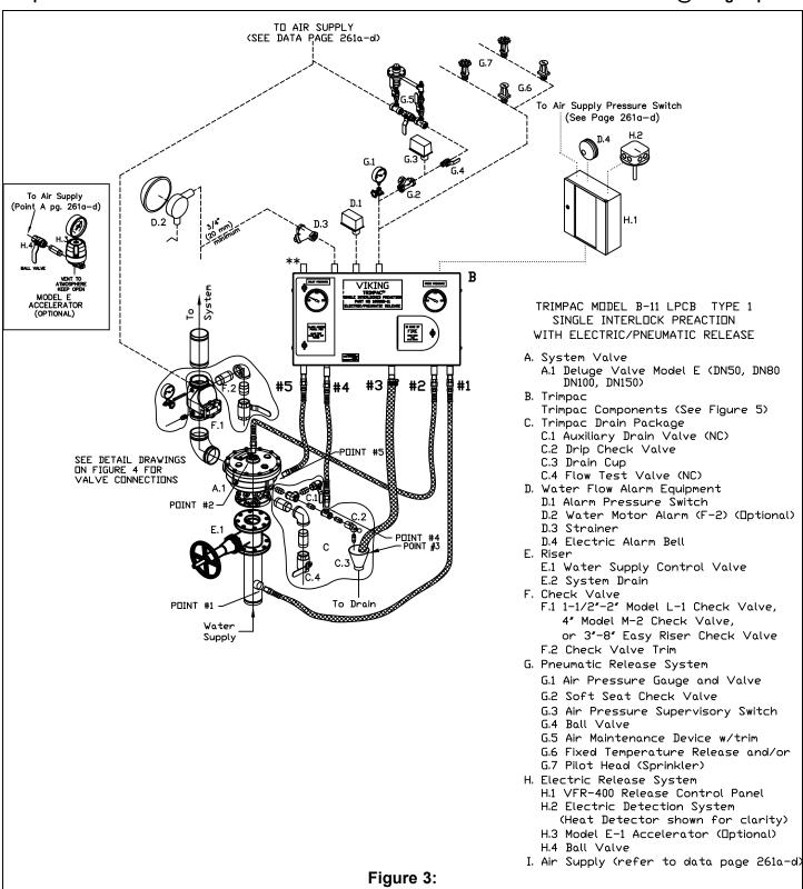
Trimpac® Single Interlock Preaction System with Electric/Pneumatic Release 2", 3", 4" & 6" (DN50, DN80, DN100, & DN150)
