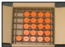
CORRECT (Protective caps in place)
