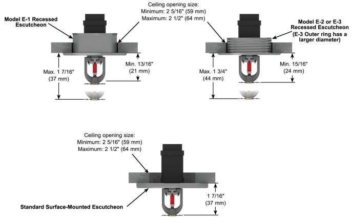
Figure – 1 Installation Dimensions with Viking Escutcheons
