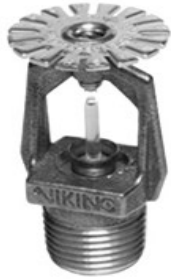
COIN® Quick Response CCombustible Interstitial Glass Bulb Upright (Specific Application) SIN: VK900 K Factor: 4.2 (60) Thread Size: 1/2 inch NPT Base Part #: 12493
