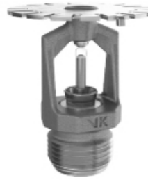
COIN® Quick Response CCombustible Interstitial Glass Bulb Upright (Specific Application) SIN: VK950 K Factor: 5.6 (80) Thread Size: 1/2 inch NPT Base Part #: 20757
