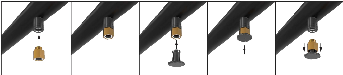
Figure 4B: Inserting Gasket into IS-W2 Fitting
