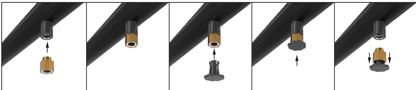
Figure 4B: Inserting Gasket into IS-W2 Fitting
