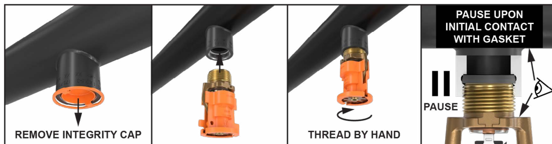
Figure 3A: Seating the Sprinkler
