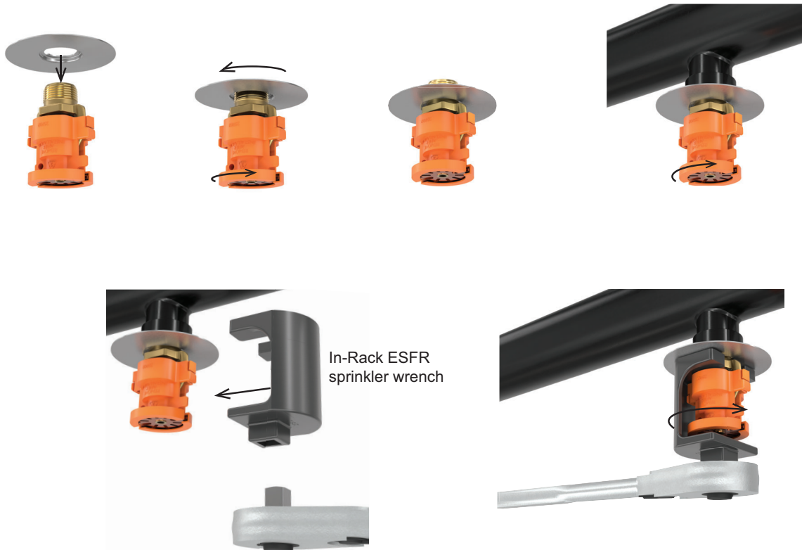
Figure – 4: Installing the ES Series Water Shield
