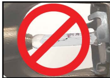
INCORRECT (bulb cracked, fluid missing)
