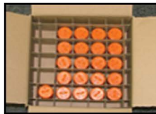
CORRECT (Protective caps in place)
