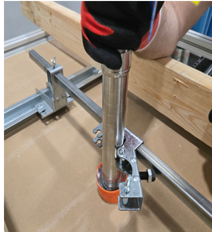
Figure – 3: Place Assembly into the Hub
