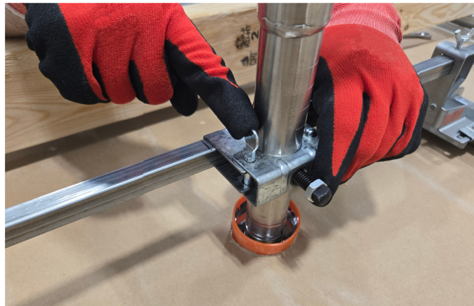
Figure – 4: Close Hinge Door and Locking Shaft
