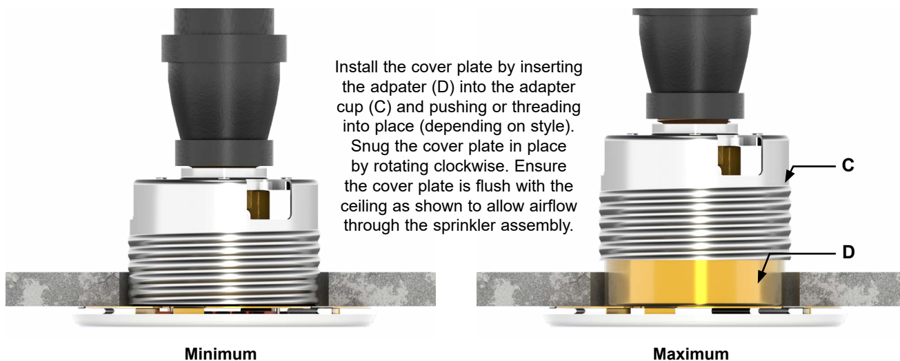
Figure 7: Installing the Cover Plate
