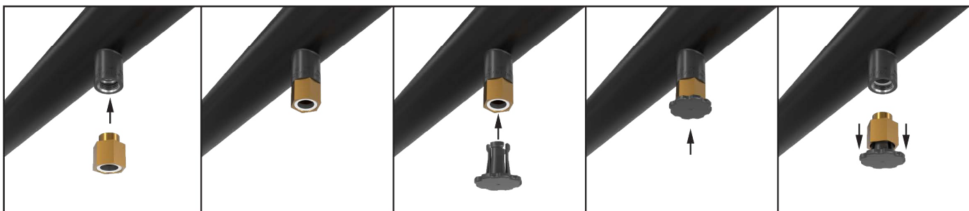
Figure 4B: Inserting Gasket into IS-W2 Fitting
