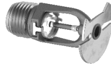
Window Sprinkler Quick Response Glass Bulb Horizontal Sidewall (Specific Application) SIN: VK962 K Factor: 5.6 (81) Thread Size: 1/2 inch NPT Base Part #: 23834
