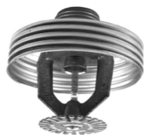
Freedom ® Residential Glass Bulb Domed Concealed Pendent SIN: VK468-D K Factor: 4.9 (71) Thread Size: 1/2 inch NPT Base Part #: 13637A-X
