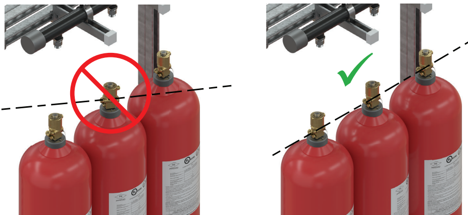
Figure 6.6: Align valve with manifold
