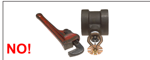
Figure 4: Incorrect installation wrench (ESFR sprinkler shown with a pipe wrench)
