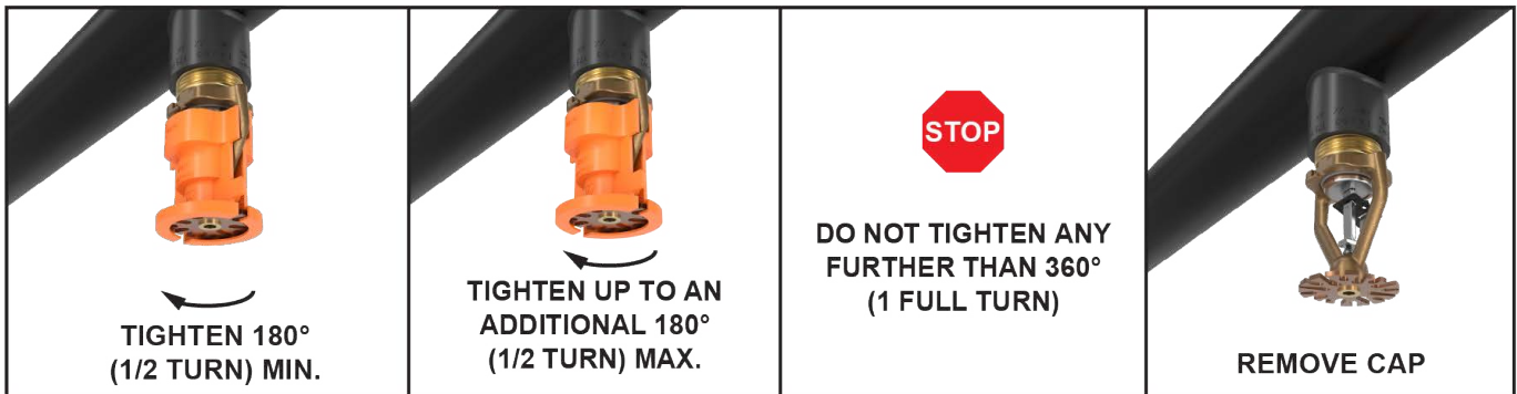
Figure 3B: Removing the Cap and Aligning the Sprinkler Frame Arms
