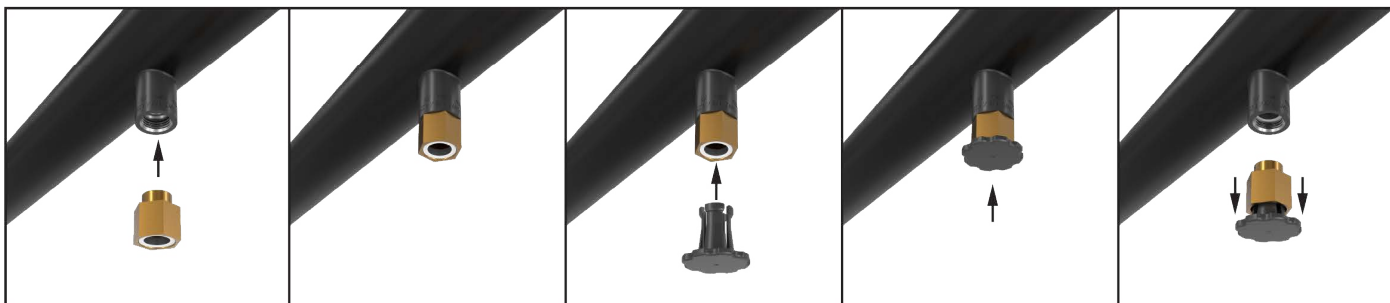
Figure 4B: Inserting Gasket into IS-W2 Fitting
