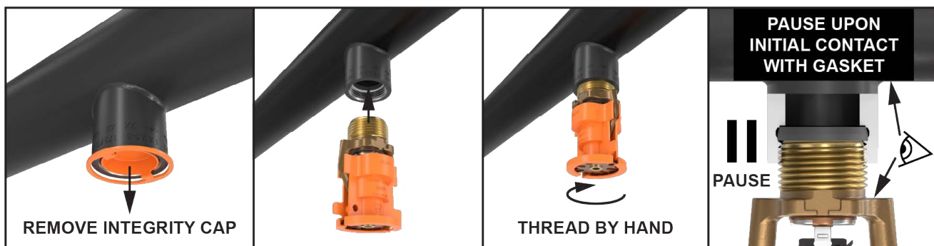
Figure 3A: Seating the Sprinkler
