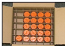
CORRECT (Protective caps in place)
