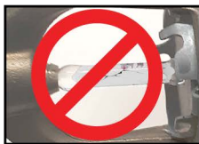
INCORRECT (bulb cracked, fluid missing)
