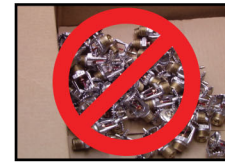
INCORRECT (Stored loose in a box)
