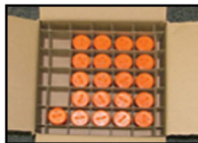
CORRECT (Protective caps in place)
